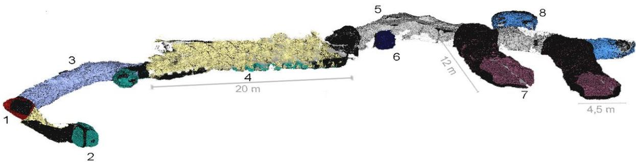
Figure 17. First battery in the cave in the lower part of *Monte Celva* (1: entrance of the structure; 2: lower casemates; 3, 5: connecting galleries; 4: rifleman emplacements; 6: guard post, 7: artillery battery in cave, 8: ammunition depot).
