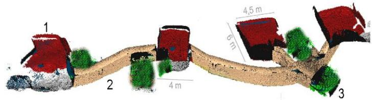
Figure 16. Fourth battery in cave: gun emplacements (1), connecting underground gallery (2), underground casemate (3).
